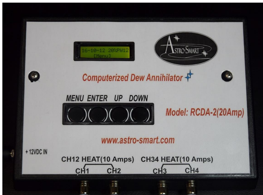
Figure 1: Computerized Dew Annihilator (RCDA-2)
